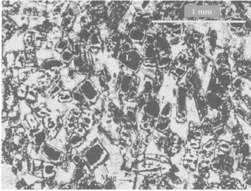
FIG. 3. Photomicrograph of B-bearing iron ore from Tallgruvan, Norberg with stubby prisms of ludwigite partly altered to a transparent B-bearing mineral and magnetite. L: ludwigite, Mag: magnetite. Sample 450514.
