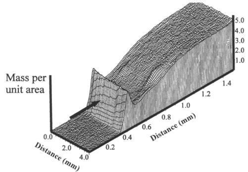
FIG. 4. SMR area scan of a developed lesion in a 200  $\mu\text{m}$  section of permeable hydroxyapatite aggregate after exposure to a 0.1 mol  $\text{l}^{-1}$  lactic acid demineralizing solution at pH 4.0 (151 points at 10  $\mu\text{m}$  intervals in the direction perpendicular to the surface, 40 points at 100 intervals in the direction parallel to the surface, 10 s per point.) The arrow indicates the direction of acid attack. (After Fig. 5.1.1.2 in Anderson, 1988).
