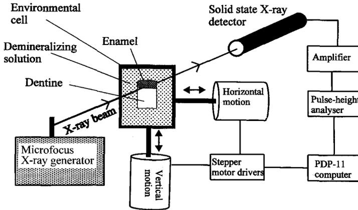
FIG. 1. Schematic of scanning microradiography (SMR) system.
