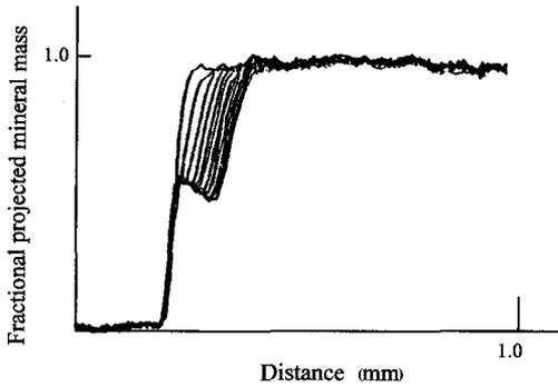
FIG. 3. Demineralization of  $\text{Ca}(\text{OH})_2$  aggregate by de-ionized water. Mo- $K_{\alpha}$  radiation, 10 s at each point, 101 points at 10  $\mu\text{m}$  intervals, scan every 3 h (from Fig. 13 in Anderson and Elliott, 1992).
