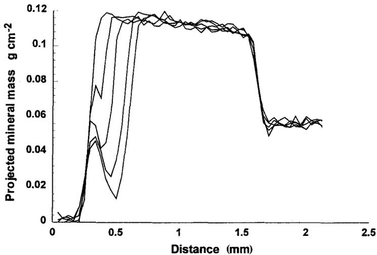
FIG. 2. Demineralization of enamel section from its natural surface by sodium acetate/acetic acid buffer at pH 4.0. Ag- $K_{\alpha}$  radiation, 10 s at each point, 100 points at 10  $\mu$ m intervals, scan every 54 h.
