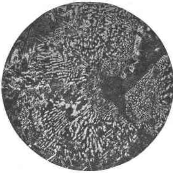
FIG. 8. Graphic intergrowth of hematite (white) and magnetite. Hematite apparently secondary. Some blades of ilmenite around edges. (Etched). Poplar Lake, Minnesota. Mag. X 125.
