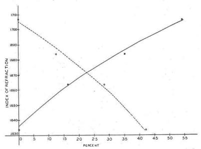
FIG. 4. Relations of refractive index and composition in the Apatite-Svabite series. Solid line, variation of refractive index ( $\omega$ ) with As<sub>2</sub>O<sub>6</sub> content. Dotted line, variation of refractive index ( $\omega$ ) with P<sub>2</sub>O<sub>6</sub> content.
