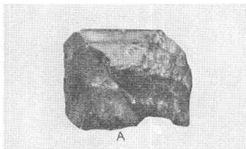
FIG. 2. Photograph showing part of monazite of Fig. 1, natural size after freeing from the rock. The front surface in the photo probably represents the top side of crystal growth seen in Fig. 1. The diagonal fracture from NW to SE seems to indicate a twinning plane between a parallel growth to the NE and a twin to the SW. The plane of fracture parallel to the surface of the paper thus appears to be common to a twin and a parallel growth. Unfortunately the part broken away from the SW front half, below the diagonal fracture, which would have given the key to the arrangement, was lost. Parallel growths are developed on the back of this mass.
