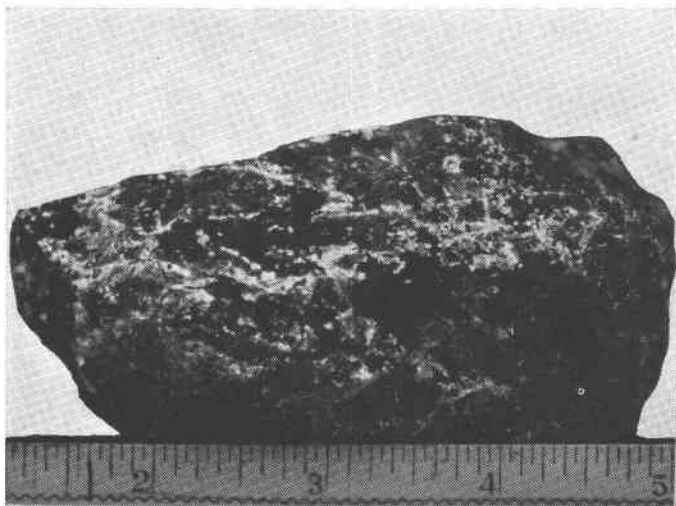
FIG. 1. Nepheline syenite from Beemerville, New Jersey, under ultra-violet light. White is fluorescent sodalite of secondary origin, occurring in veinlets and in zones surrounding cores of nepheline.
