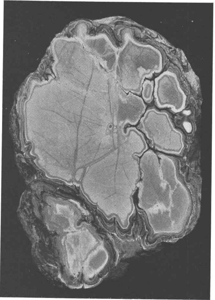
FIG. 1. Photograph of a polished variscite nodule. The black seams are fine-grained quartz; the gray seams in the center of the nodule are a darker green variscite in a normal variscite. The white shell surrounding the variscite is a dense pseudowavellite; the outer finely-banded material is the early pseudowavellite. \times 1
