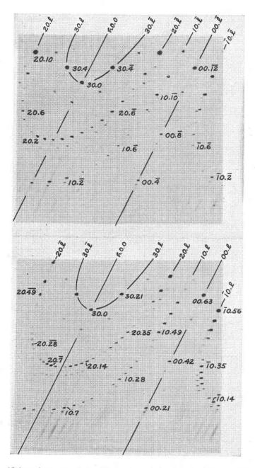
FIG. 15 (upper). Equi-inclination Weissenberg photograph of  $\alpha$ -SiC, type III; a-axis rotation, zero level.
