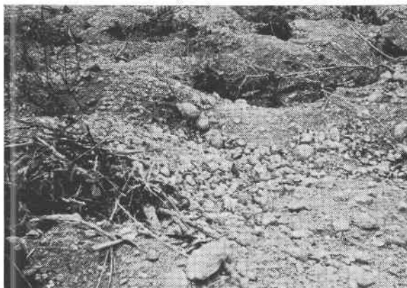
FIG. 10. Eluvial deposit, northwest of Sete Lagôas, Minas Gerais. Crystals are picked from the dirt which is broken down by picks and shovels. A carry-all removes the material to the dump.
