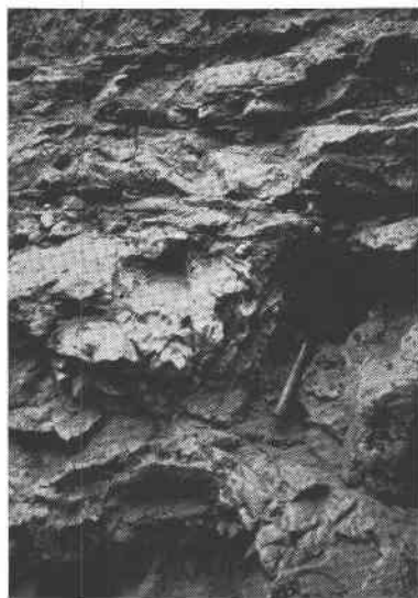
FIG. 7. Blanket deposit. Mimoso, Baia. Coarse-grained bull quartz and pockets from which commercial crystal has been removed.
