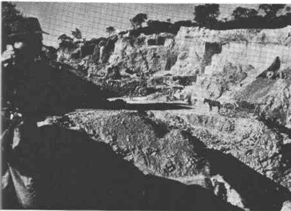
FIG. 3. Looking south along strike of the vein zone, Onca Mine, Sete Lagôas, Minas Gerais. Weathered shale to the right is the hanging wall. Footwall of granite is in shadow to the left.
