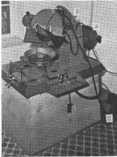
FIG. 2. Felker saw mounted on concrete block. (A) Adjustable counterweight; (B) depth stop; (C) coolant tank and circulating pump.
