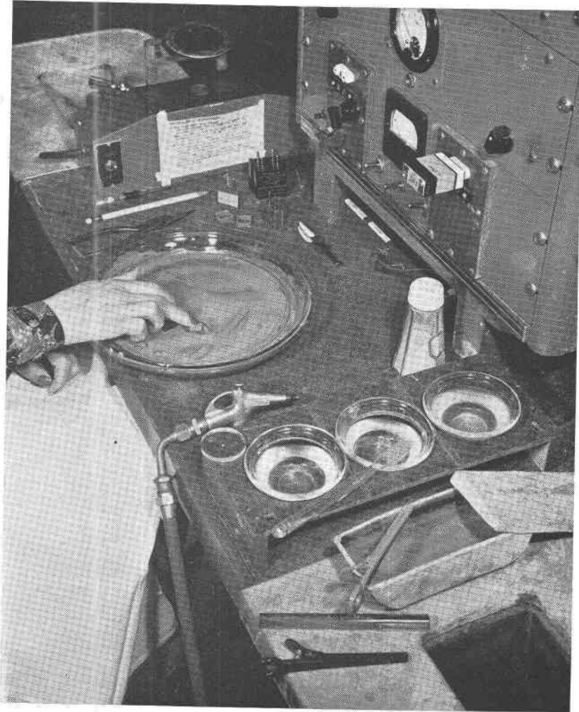
FIG. 1. Final abrasive finishing position, showing glass lap (held in a pie dish) with crystal and abrasive, comparison oscillator with standard crystal, polariscope (left) for determining X and Z' directions, sink with soap solution and tooth brush for cleaning, air gun for drying, and lead dish of etching solution with plastic holding tongs for acid wash.
