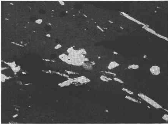
FIG. 9. Fluorite (gray ground mass) replacing sulfides (black) and quartz (white equidimensional areas). Sericite (white laths) cuts fluorite and sulfides; nicols at 45^\circ ; \times 45 .
