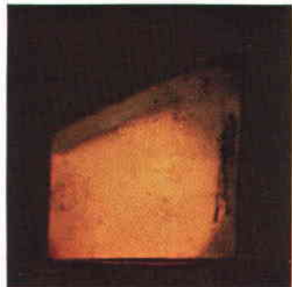
FIG. 2. ( right ) Phosphorescent specimen of spodumene after irradiation, illuminated only by its own phosphorescence.
