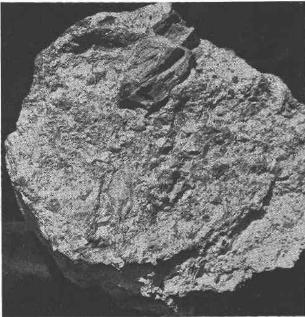
FIG. 4. Fresh surface of Peña Blanca Spring meteorite. The large crystal, about 2.5 inches long is enstatite. The oval black spot at end of crystal is metal and sulfide.
