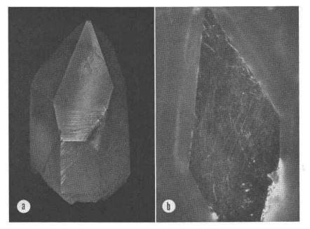
FIG. 1. (a) Natural quartz crystal in white light. (b) Autoradiograph caused by adsorbed Cs<sup>137</sup>.
