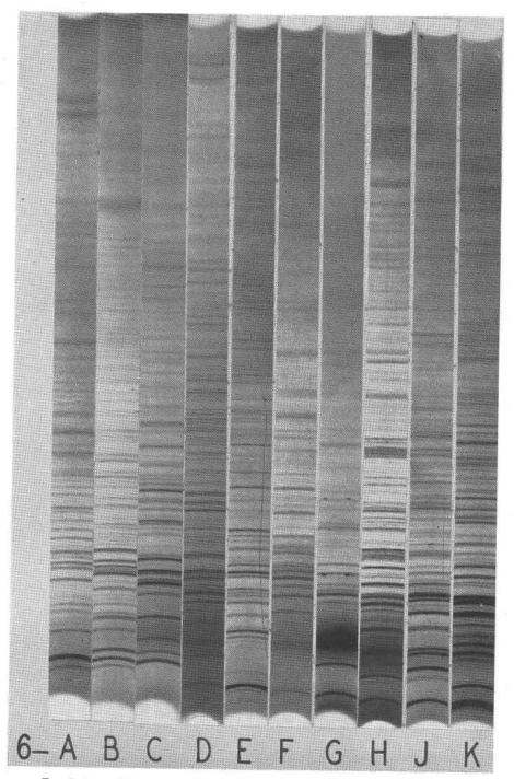
FIG. 6. X-ray diffraction patterns for phosphates whose strongest line corresponds to d of 6.5 to 10.5 Å.
