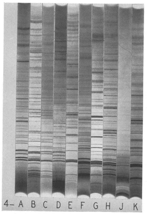
FIG. 4. X-ray diffraction patterns for phosphates whose strongest line corresponds to d of 3.18 to 3.40 Å.
