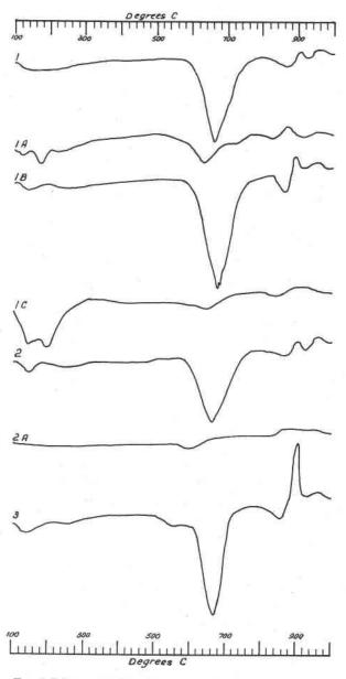
FIG. 1. Differential thermal curves of chlorite and associated minerals from Cobargo, N.S.W.
