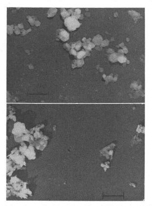
FIG. 4. Electron micrographs of kaolinite samples 0-34-15 (above) and V-56-200, (below) showing the difference in crystallization. Pd-shadow.
