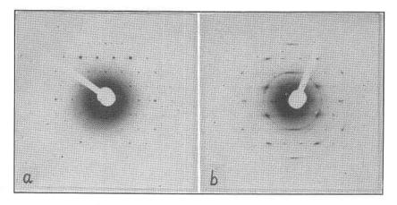
FIG. 2. Single crystal electron diffraction patterns of sepiolite from (a) Little Cottonwood, Utah, (b) Eski Chehir, Asia Minor.
