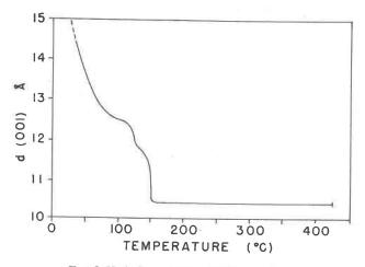
FIG. 3. Variation of (001) with temperature.
