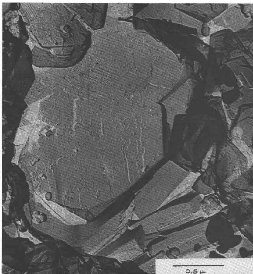
FIG. 3. H 2 SO 4 -treated kaolinite showing reaction product "chains" on basal surfaces. \times 76,000 .
