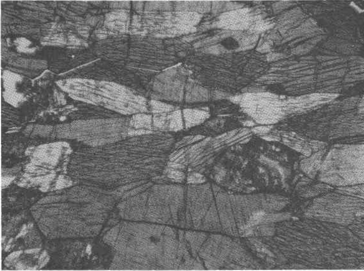
FIG. 1. Cummingtonite-bearing amphibolite from Duchess, Queensland, showing hornblende (shades of gray), cummingtonite (colorless), and heavily altered plagioclase. The cummingtonite occurs mainly as independent grains, but also as composite grains with hornblende. Lamellae parallel to (001) of cummingtonite in an independent hornblende grain (bottom) and a hornblende-cummingtonite composite grain (left-center) appear as "striations" at this magnification. Plane-polarized light ( \times 35 ).
