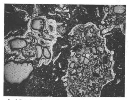
Fig. 5. Photomicrograph. Manganiferous fragments in barren material. Thin concretionary rims of manganese oxide are intact within fragments and broken outside of fragments.  $120\times$ .
