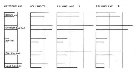
FIG. 2. Semi-quantitative partial x-ray spectrographic analyses. The horizontal lines represent the maximum peak values obtained for a particular spectral line of the element indicated. Two partial analyses of each mineral are given. Distance between vertical lines is equal to one-fourth of the x-ray spectrograph scale. A LiF analyzing crystal was used and all reflections are first order.
