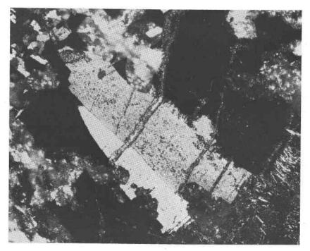
FIG. 1. Photomicrograph. Large cryptomelane grains that occur interlayered with jasper in the Black Jack deposit. The cloudy and unevenly highlighted gray and white material is quartz. Partial outlines of quartz crystals may be seen in places along the edges of the cryptomelane grains.  $370 \times$ . Crossed nicols.
