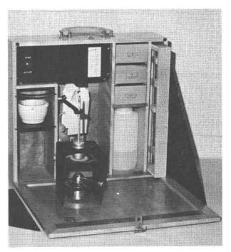
Fig. 1. Photograph of zeolite test kit.
