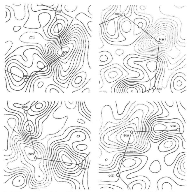
Fig. 4. Difference density maps. Contours at 0.05 e/A<sup>3</sup>; negative contours dotted. The sections shown lie in the plane of the boron and two oxygen atoms. The solid lines indicate bonds lying in the section.
