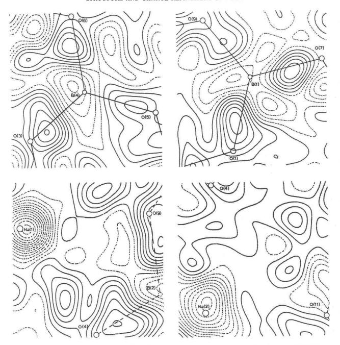
Fig. 5. Difference density maps. Contours at  $0.05 \text{ e/A}^3$ ; negative contours dotted. The sections in the upper half of the figure contain the three oxygen atoms, while those in the lower half are through one sodium and two oxygen atoms. The solid lines indicate bonds lying in the section; the dashed lines are projections of bonds to atoms not lying in the plane of the density map.
