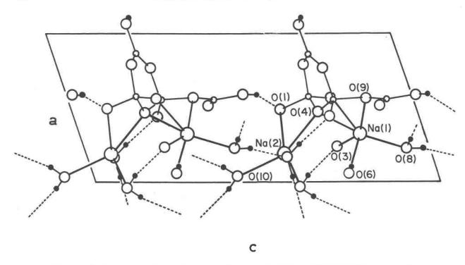
Fig. 3. Projection of the structure on the ac plane showing the hydrogen bonding and sodium coordination.
