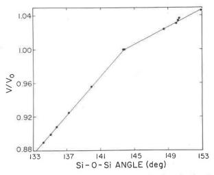
Fig. 10. The Si–O–Si angle of quartz as a function of unit-cell volume at temperature or pressure normalized to room-pressure-temperature volume. The break in slope at the room-temperature-pressure point suggests that different structural changes cause the volume change for increased temperature or pressure.
