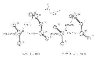
Fig. 2. The effect of pressure on the cavities in the quartz structure. The Si-O-Si angle compresses from  $143.73^{\circ}$  at 1 atm to  $134.2^{\circ}$  at 61.4 kbar. The shortening of two long O-O interatomic distances shown in this figure appears to be partially responsible for the difference in compressibilities along the *a* and *c* crystallographic directions.
