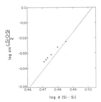
Fig. 9. Plot of log d(Si  $\cdots$  Si) vs. log sin[Si–O–Si)/2] for the silica polymorphs. The line represents the trend shown in Hill and Gibbs (1979) for the silica minerals measured under ambient conditions. The crosses represent the data for quartz from this study, measured at six pressures including room pressure. This relationship may hold for general P-T conditions.
