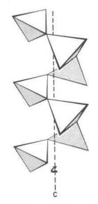
Fig. 12. Spirals of silicate tetrahedra parallel to c. These easily expanding and contracting spirals behave like coiled springs and are, therefore, responsible for the low value of Poisson's ratio in quartz.
