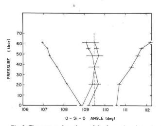
Fig. 3. The pressure dependence of the four unique internal tetrahedral angles (O-Si-O).
