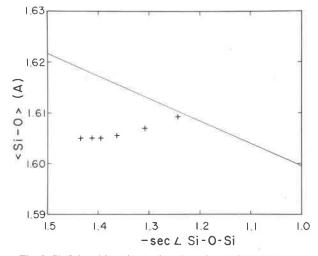
Fig. 8. Si-O bond length as a function of -sec(Si-O-Si) for the silica minerals. The line represents the trend shown in Hill and Gibbs (1979) for the polymorphs measured under ambient conditions; the crosses represent the data for quartz from this study at six pressures, including room pressure. This relationship does not persist at high pressure.
