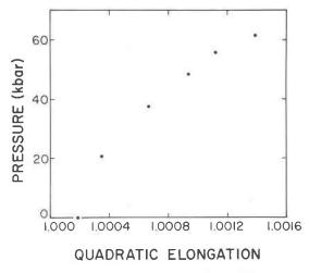
Fig. 4. Increase in tetrahedral distortion with pressure as indicated by quadratic elongation. The curvature of the data indicates that the amount of distortion per kbar is greater at higher pressures than at lower pressures.
