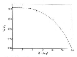
Fig. 11. The tetrahedral tilt parameter for quartz,  $\delta$ , as a function of unit-cell volume at temperature or pressure normalized to the room-temperature-pressure volume. The hyperbolic shape of this curve suggests that tetrahedral tilting is important to the change in unit-cell volume as the  $\alpha$ - $\beta$  transition is approached but has less effect as unit-cell volume decreases.
