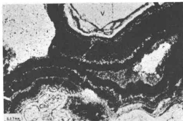
Fig. 2. Photomicrograph of theophrasite, dark, covering idocrase (V) and chlorite (Chl), cross section, Vermion.
