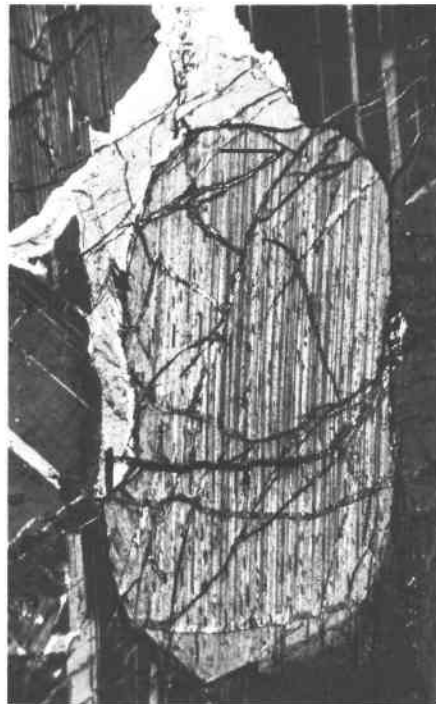
Fig. 3. Photomicrograph of type 1 (Bushveld-type) exsolution in leuconorite sample PL-150. Exsolution consists of fine (100) augite and parallel Fe-Ti oxide minerals. Scale bar is 0.10 mm.
