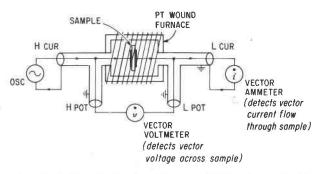
Fig. 1. Schematic drawing of the experimental setup denoting the four-terminal pair assembly. H and L refer, respectively, to the high and low leads of the current or potential connections.
