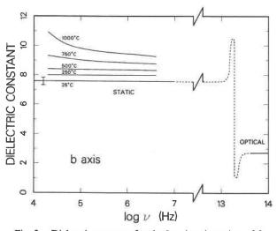
Fig. 2. Dielectric constant for the **b**-axis orientation of forsterite determined at selected temperatures as a function of the logarithm of the electric-field frequency. Error bar denotes the measurement uncertainty in the dielectric constant.
