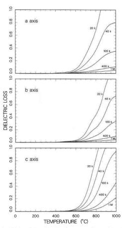
Fig. 4. Dielectric loss for the three crystallographic orientations of forsterite measured at selected frequencies as a function of temperature. Frequency labels are in units of hertz. The loss data have a relative uncertainty of approximately 5%.
