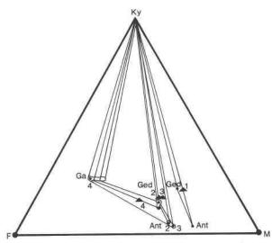
Fig. 11b. Chemographic relations of the phases anthophyllite (Ant), gedrite (Ged), kyanite (Ky), and garnet (Ga) in the orthoamphibole zone as shown in an A'FM diagram. Garnet unstable in Mg-rich compositions. 1 = DV1, 2 = DV43, 3 = DV22, 4 = DR184,  $\triangle$  = composition of sample.
