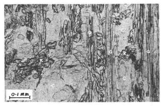
Fig. 6b. Hydration of cordierite (C) along isograd (sample M346). G = gedrite.
