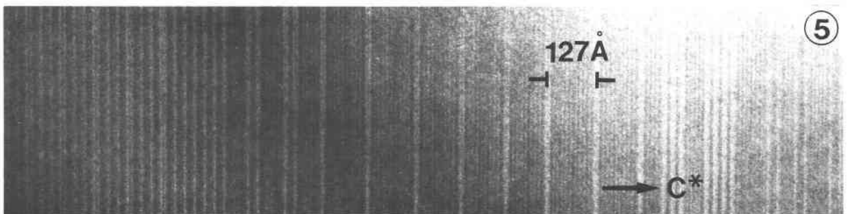
Fig. 3 (upper photograph). An ordered sequence of twinning in leucophoenicite resulting in a superperiodicity with d_{(001)} = 165 \text{ \AA} .
