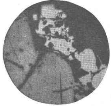
FIG. 2. Passed thru 20-mesh screen. White, pentlandite; gray, pyrrhotite; black, gangue and wax. Magnification 150 \times .
