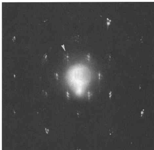
FIGURE 7. Six star-like arrangements of satellite reflections on the antigorite 020- and 110-type subcell reflections. This is diagnostic of k \times 60^\circ rotation of twin individuals. Twin individuals are superimposed along c^* owing to modulation fringes crosscutting each other as visible in Figure 6.
