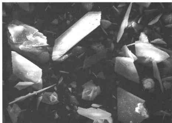
FIGURE 2. SEM of hydroxylapatite (HAP) reactant used in batch sorption experiments showing plate-like particles of various sizes (image size = 570 \times 410 \mu\text{m} ).
