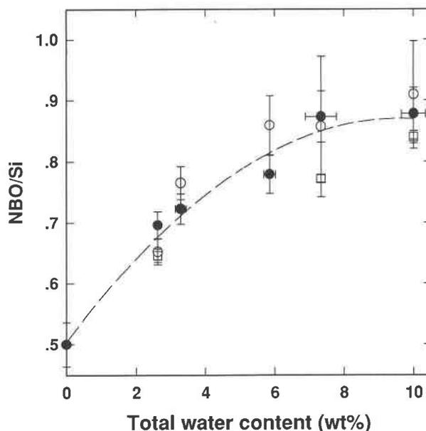
FIGURE 11. Dependence of the number of non-bridging O atoms per silicon (NBO/Si) on the total water content: Raman data (empty circles); NMR data (empty squares); and near IR data (full circles). The dashed line is a polynomial fit through all the data points.
