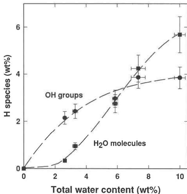
FIGURE 10. Dependence of the concentration of OH groups and H<sub>2</sub>O molecules in hydrous sodium tetrasilicate glasses on the total water content. The dashed lines are a guide for the eyes only.
