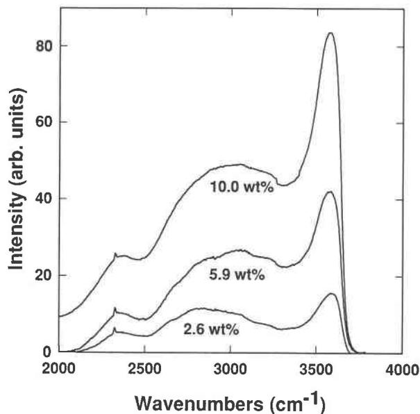
FIGURE 13. Unpolarized Raman spectra of hydrous sodium tetrasilicate glasses in the OH stretching region ( $2000\text{--}4000\text{ cm}^{-1}$ ). The sharp feature at about  $2325\text{ cm}^{-1}$  is due to  $\text{N}_2$  in the air.
