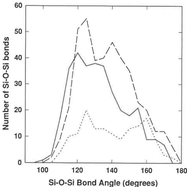
FIGURE 7. Distribution of Si-O-Si bond angles for different  $\text{Q}^n$ - $\text{Q}^m$  species according to a model of the anhydrous sodium tetrasilicate glass obtained by reverse Monte Carlo simulations:  $\text{Q}^4$ - $\text{O}$ - $\text{Q}^4$  (full line),  $\text{Q}^4$ - $\text{O}$ - $\text{Q}^3$  (dashed line),  $\text{Q}^3$ - $\text{O}$ - $\text{Q}^3$  (dotted line).
