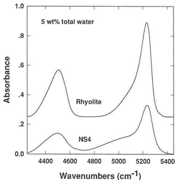
FIGURE 15. Near IR spectra of synthetic, iron-free rhyolite glass and of sodium tetrasilicate glass (NS4). Total water content in both samples 5 wt%, spectra normalized to 1 mm thickness.
