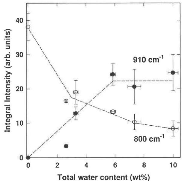
**FIGURE 5.** Integral intensity of the 800 (open circles) and 910 (filled circles) cm<sup>-1</sup> band in the reduced unpolarized Raman spectra as function of total water content. The dashed lines are a guide for the eyes only.
