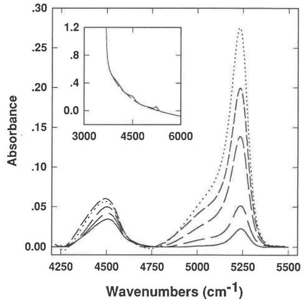
FIGURE 8. Baseline-corrected near IR spectra of hydrous sodium tetrasilicate glasses with 2.62 wt% total water (full line), 3.29 wt% (long-dash line), 5.86 wt% (medium-dash line), 7.34 wt% (short-dash line) and 10.0 wt% (dotted line). All spectra are normalized to  $450 \mu\text{m}$  thickness. The inset shows the raw spectrum (full line) of the sample with 3.29 wt% total water together with background (dashed line).
