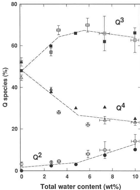
**FIGURE 4.** Dependence of the Q-species distribution in hydrous sodium tetrasilicate glasses on the total water content: Q<sup>2</sup> (circles), Q<sup>3</sup> (squares), Q<sup>4</sup> (triangles). Raman data (open symbols), NMR data (filled symbols). The dashed lines are only a guide for the eyes.
