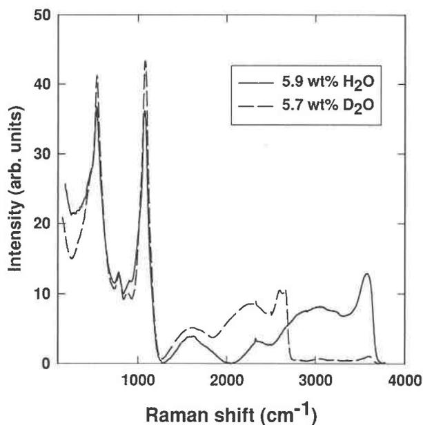
FIGURE 14. Unpolarized Raman spectra of the hydrous sodium tetrasilicate glass with 5.9 wt%  $\text{H}_2\text{O}$  and the deuterated glass with 5.7 wt%  $\text{D}_2\text{O}$ . The two spectra are normalized so that the area of both curves in the range  $150\text{--}1300\text{ cm}^{-1}$  is the same.
