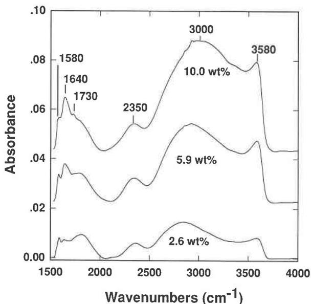
FIGURE 12. IR spectra of hydrous sodium tetrasilicate glasses in the OH stretching region ( $2000\text{--}4000\text{ cm}^{-1}$ ). Spectra are offset by 0.02 absorbance units for clarity. All spectra are normalized to  $450\text{ }\mu\text{m}$  thickness.
