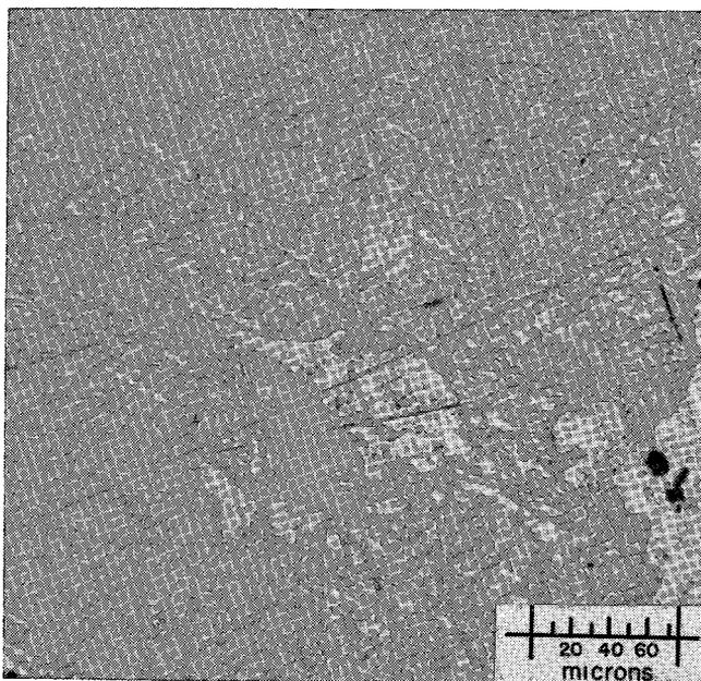
FIG. 1. Photomicrograph of a polished section showing the texture of silver-antimony minerals in the Cobalt ores. The white irregular areas and white lamellae represent phase 1. The light grey area forming the main part of the photograph represents phase 2, and the dark grey areas around phase 2 as well as the lamellae in phase 2 represent phase 3 (allargentum). (This photograph was taken in oil immersion to enhance contrast.)
