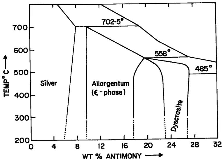
FIG. 2. Phase equilibrium diagram of the silver-rich end of the Ag-Sb system (from Somanchi 1966, slightly modified by the authors).
