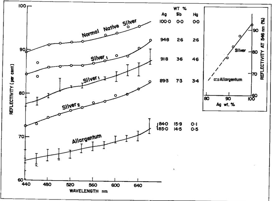
FIG. 3. Reflectivity spectra of silver and allargentum from Cobalt. The graph in the upper right-hand corner shows the relationship between reflectivity of these minerals at 546 nm and the weight per cent silver.
