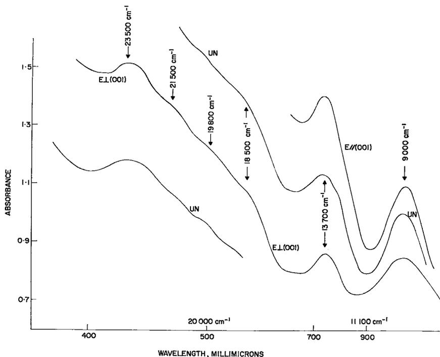
FIG. 3. Polarized ( $E_{\parallel}(001)$  and  $E_{\perp}(001)$ ) and unpolarized (UN) spectra of black tourmaline from Villeneuve, Labelle County, Quebec, using a specimen 0.011 cm thick (the two UN curves are the result of using different scale factors for the two ends of the spectrum).
