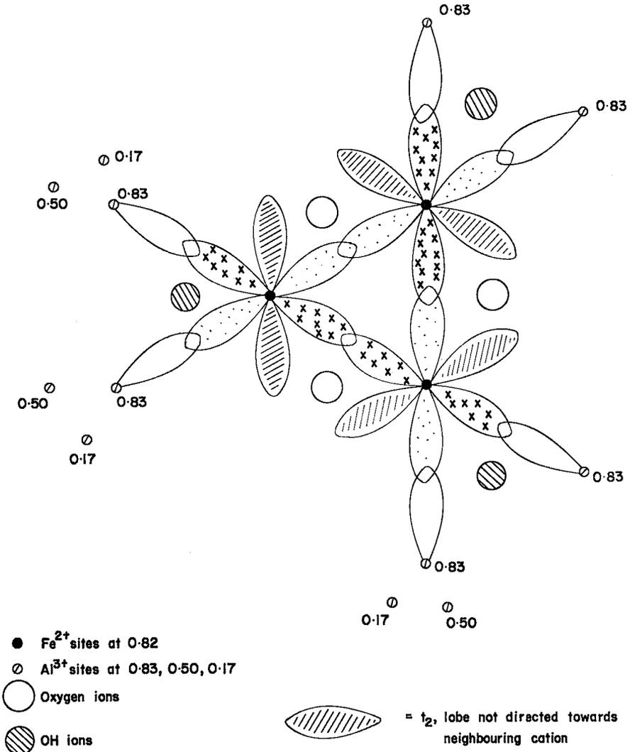
FIG. 1. Diagrammatic representation of the structure of tourmaline projected on (001) showing the relationship between octahedral sites in spiral chains (small crossed circles at heights of 0.83, 0.50 and 0.17) and brucite units (black circles at a height of 0.82) The  $d_{z^2}$  orbital lobes lying in the 001 plane are shown as balloon-shaped envelopes for the cations in the trigonal units, and for a few of those in the spiral chains.
