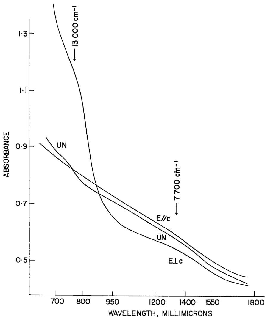
FIG. 5. Polarized ( $E//c$  and  $E\perp c$ ) and unpolarized spectra of buergerite, using a specimen 0.002 cm thick.
