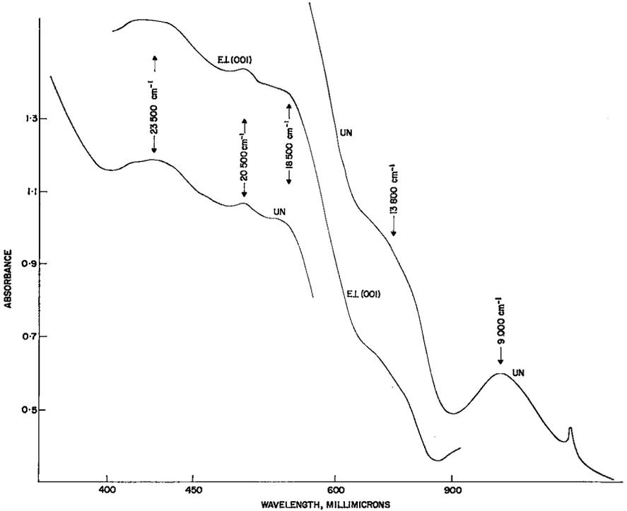
FIG. 4. Polarized ( $E\parallel(001)$ ) and unpolarized (UN) spectra of black tourmaline from Como, Italy, using a specimen 0.025 cm thick (two different scale factors were used for the unpolarized spectrum).
