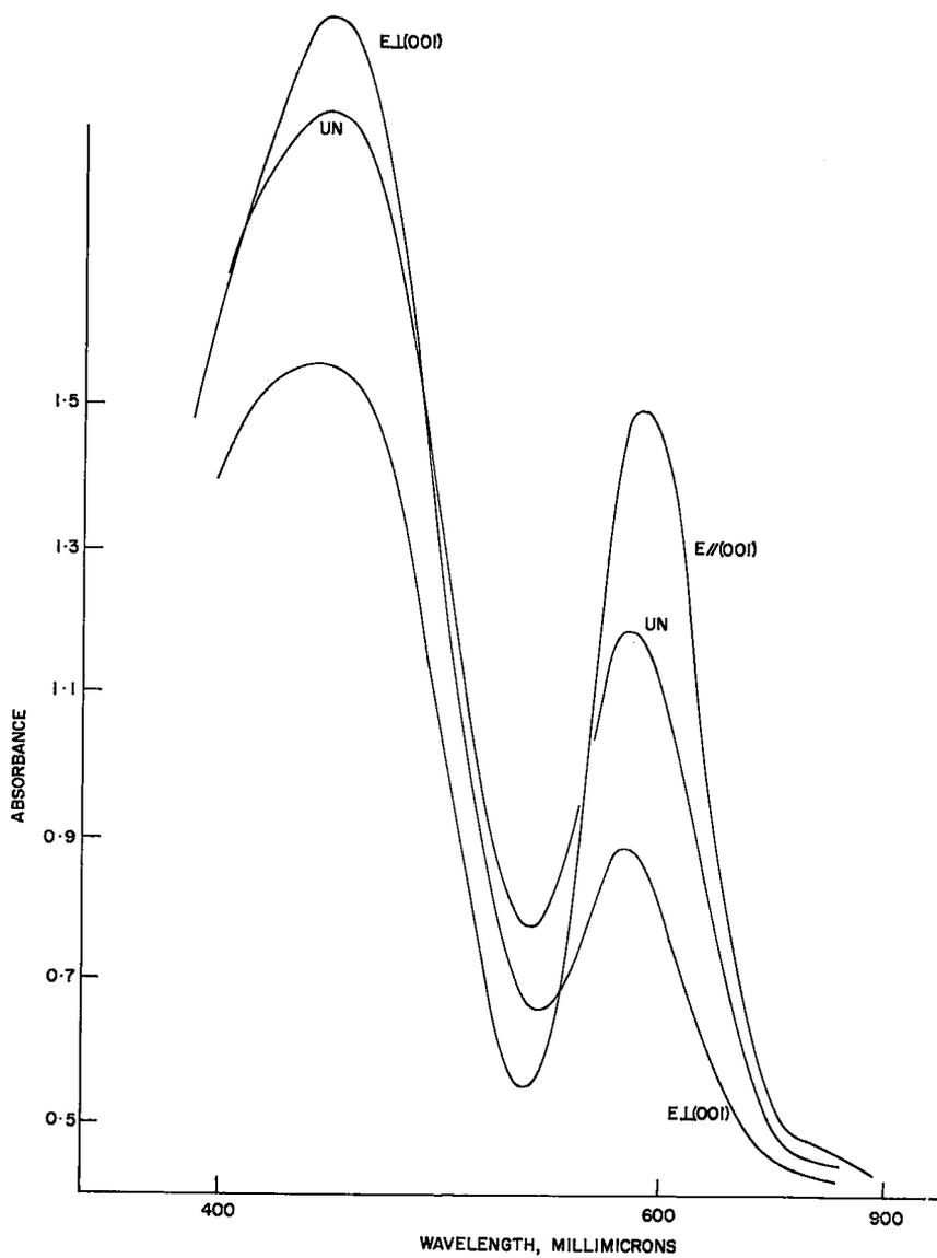
FIG. 2. Polarized ( $E_{\perp}(001)$  and  $E_{\parallel}(001)$ ) and unpolarized (UN) spectra of Cr-bearing tourmaline, using a specimen 0.005 cm thick.
