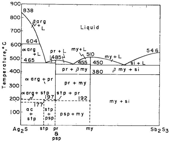
FIG. 147. Pseudobinary system Ag<sub>2</sub>S-Sb<sub>2</sub>S<sub>3</sub> (from Keighen & Honea 1969). All assemblages are in equilibrium with vapour. *arg* = argenite, *pr* = pyrargyrite, *stp* = stephanite, *ac* = acanthite, *psp* = pyrostilpnite, *my* = miargyrite, *si* = stibnite. The dotted lines indicate the uncertainty of low temperature relations. Both stephanite and pyrostilpnite have never been synthesized, and the pyrargyrite-pyrostilpnite reaction has not been established.
