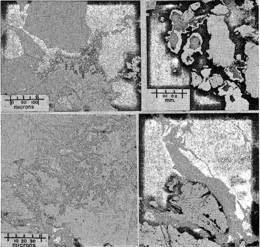
FIG. 142. (Top, left) Irregular grain of stromeyerite (grey) with pearceite (111) (lighter grey at centre of photograph). A grain of chalcopyrite (white) is present in calcite (black) at extreme right of photograph. (Morrison mine, sample M-16326).
