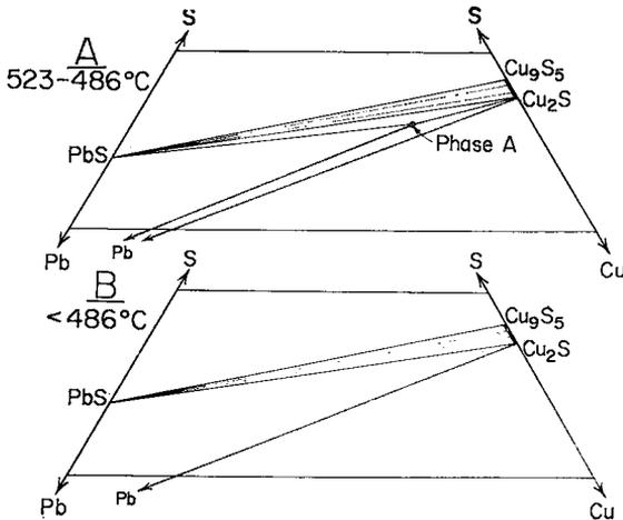
FIG. 141. Portions of the Cu-Pb-S ternary system below  $486^\circ\text{C}$  and at  $486-523^\circ\text{C}$  (from Craig & Kullerud 1968). Phase A is shown in the top illustration but not in the lower one.
