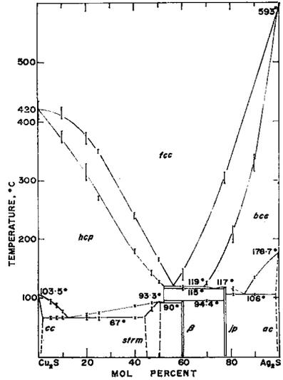
FIG. 140. Binary section of the  $\text{Cu}_2\text{S}-\text{Ag}_2\text{S}$  system (from Skinner 1966). *ac* = acanthite, *bcc* = body centered cubic, *cc* = chalcocite, *fcc* = face centered cubic, *hcp* = hexagonal close packed, *jp* = jalpaite, *strm* = stromeyerite,  $\beta$  = mckinstryite ( $\text{Cu}_{0.8}\text{Ag}_{1.2}\text{S}$ ). All phases co-exist with vapour.
