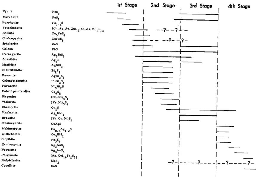
FIG. 162. Generalized paragenetic sequence for the sulphides in veins in the Cobalt-Gowganda ores. The most abundant minerals are indicated with heavy lines.
