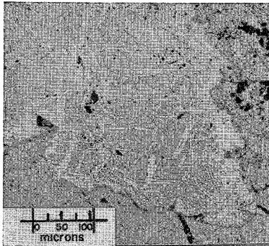
FIG. 161. A cobalt pentlandite-siegenite grain in cryptocrystalline pyrite-marca-site. The cobalt pentlandite (white) is present as lamellae in siegenite (light grey). The cobalt pentlandite-siegenite is partly bordered by a thin rim of bravoite (dark grey). (Langis mine, sample 329).
