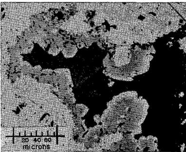
FIG. 159. A coating of layered bravoite (grey) on arsenides (white). A cobalt-rich bravoite (dark grey) is next to the arsenides, and an iron-rich one (light grey) borders it. (Langis mine, sample 329).
