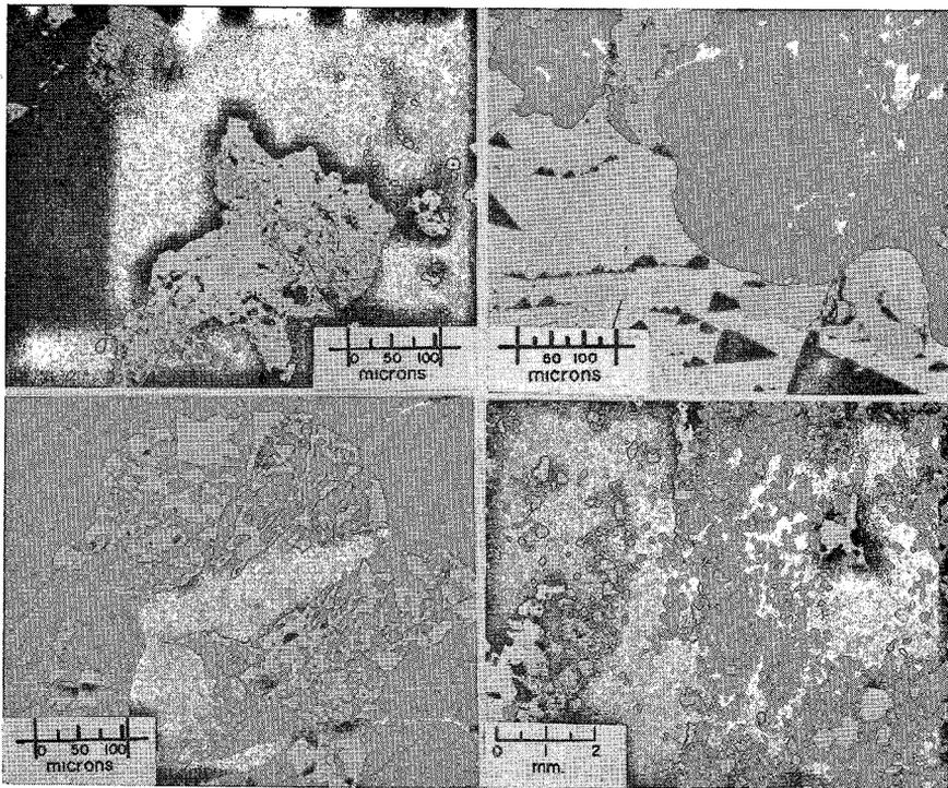
FIG. 129. (Top, left) Sulphide grain in calcite, showing chalcopyrite (dark grey) intergrown with marcasite (white). (Langis mine, sample 80).
