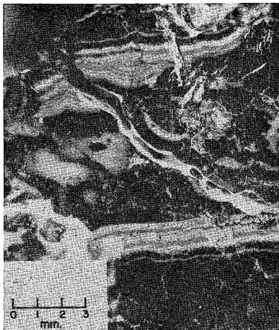
FIG. 153. Colloform sphalerite bands in a late vein. (Silverfields mine, sample 141). Photomicrograph taken by oblique illumination.
