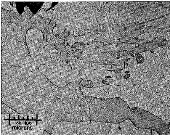
FIG. 138. Chalcocite (light grey) intergrown with stromeyerite (grey) and cut by feather-like grains of larosite. (Foster mine).
