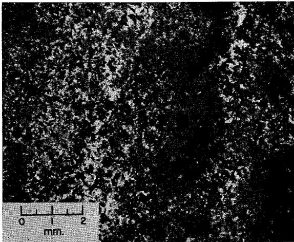
FIG. 152. Disseminated galena (white) and sphalerite (grey) at tops of slate beds in Huronian sediments. The tops of two beds are shown. (Silverfields mine, sample 763).
