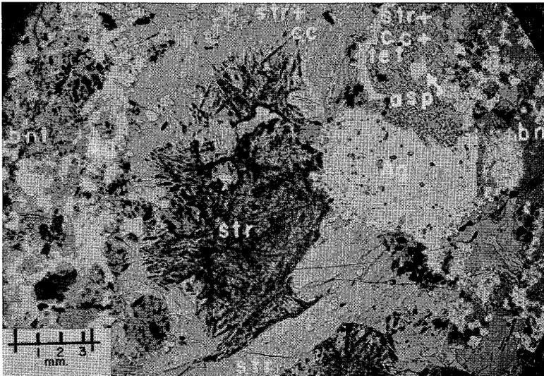
FIG. 137. Photomicrograph showing the full width of sulphide vein. It is composed of bornite (*bnt*) intergrown with silver (*Ag*) at the edges (see Fig. 136); chalcocite intergrown with stromeyerite at the centres (*str* + *cc*), and tetrahedrite (*tet*) partly replaced by chalcocite and stromeyerite (see Fig. 133). (Foster mine).
