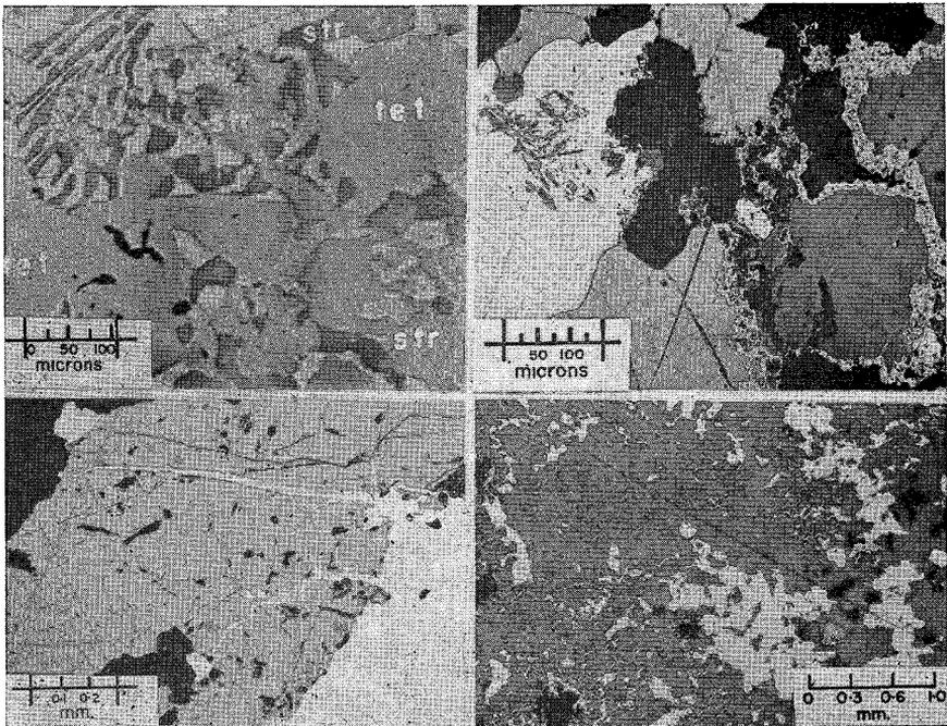
FIG. 133. (Top, left) Tetrahedrite (*tet*) remnants in a chalcocite (*cc*) - stromeyerite (*str*) intergrowth. (Foster mine).
