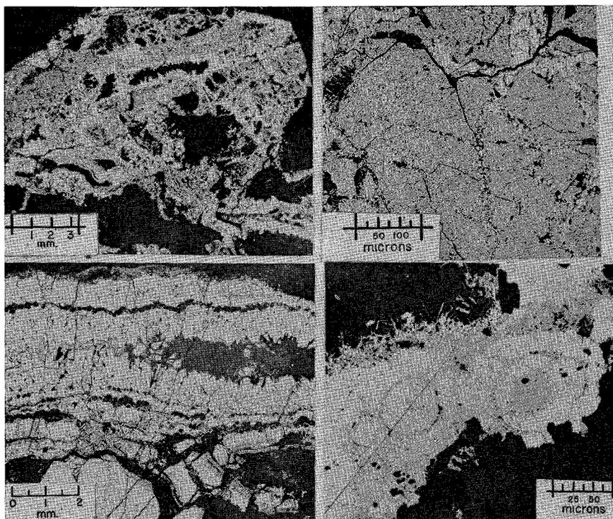
FIG. 154. (Top, left) Intergrowth of sooty-textured cryptocrystalline pyrite and marcasite (light grey area), partly bordered by marcasite crystals (white). (Langis mine, sample 89).
