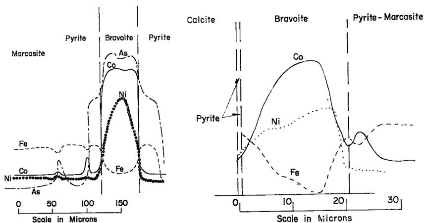
FIG. 158. Electron microprobe scans (left) for cobalt (Co), nickel (Ni), iron (Fe), and arsenic (As) across the bravoite in the concentrically-zoned grains (sample 365) (Fig. 157); and (right) bravoite in layers outside the pyrite-marcasite intergrowth (sample 329) (Fig. 159).
