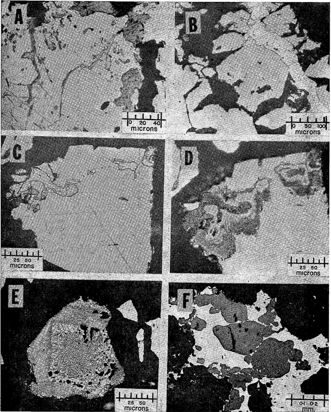
FIG. 6A. Acanthite (grey) and galena (light grey) in pyrite and arsenopyrite (white, unresolved on this photograph).
