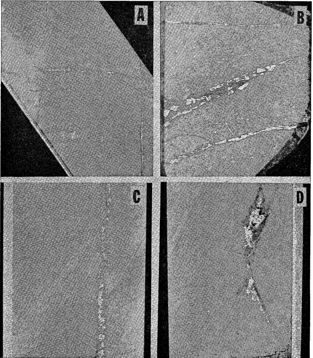
FIG. 5A. Polished face of a drill core (2.75 cm wide) showing mineralized bedding plane veins terminated by mineralized cross-veins.
