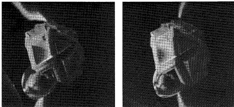
FIG. 1. SEM stereophotograph of a fourling of hexagonal \text{BaTiO}_3 . The diameter of the cuboctahedrally shaped composite is 0.3 mm.
