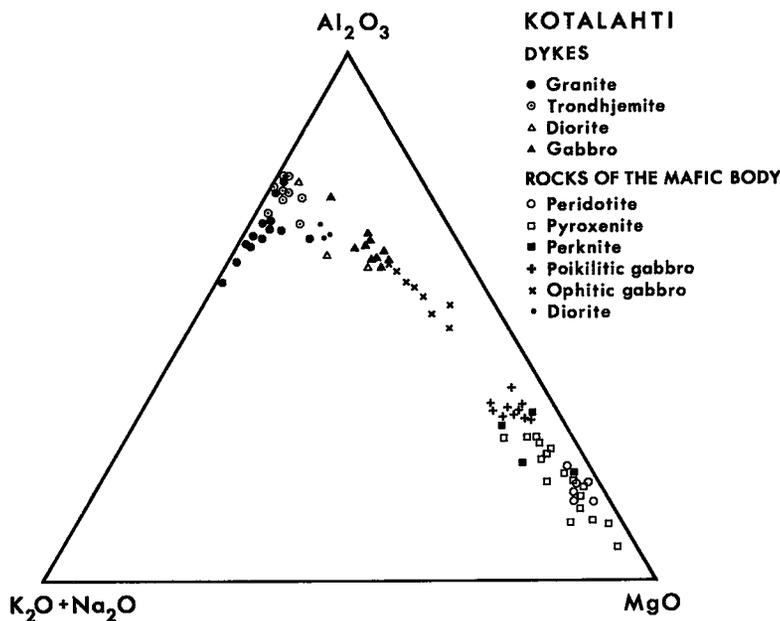
FIG. 5.  $(Na_2O+K_2O)-Al_2O_3-MgO$  plot of compositions or rock types in the Kotalahti intrusion.
