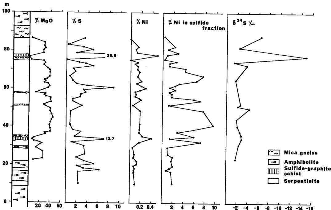
FIG. 14. A section of a serpentinite body at Siettelöjoki depicting variation in rock types, MgO (calculated on dry weight basis), Ni, S,  $\delta^{34}S$  and the nickel percentage in sulfide phase.
