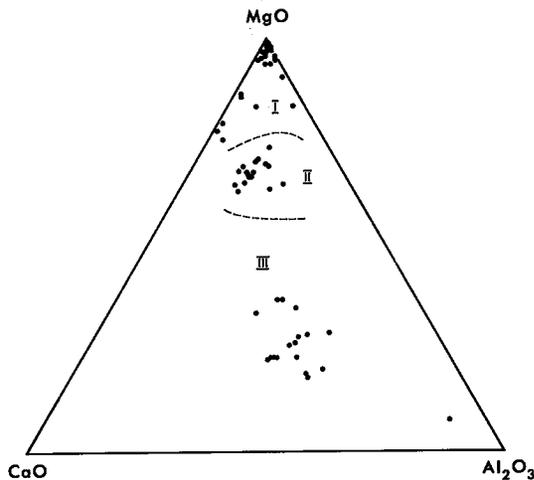
FIG. 11. MgO-CaO-Al<sub>2</sub>O<sub>3</sub> diagram showing compositions of WISB serpentinites and metaperidotites (I), cortlandites (II) and amphibolites (III).
