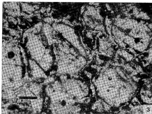
FIG. 3. Photomicrograph of magnesite pseudomorphs after equant primary olivine. Very fine-grained magnetite occupies fractures and outlines the margins of the original olivine grains. Sample 65-302. Scale bar 0.1 mm.
