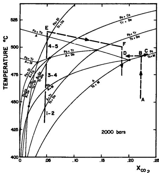
FIG. 8. Calculated T-X(CO<sub>2</sub>) phase diagram for antigorite (A), talc (Tc), tremolite (Tr), diopside (Di), forsterite (Fo), calcite (Cc), dolomite (Do) and magnesite (M) in the system CaO-MgO-SiO<sub>2</sub>-H<sub>2</sub>O-CO<sub>2</sub> (from Trommsdorff & Evans 1977). Vertical bars 1-2, 3-4, 4-5 are stable assemblages at Dumbarton (Juhas 1973). For points A, B, C, D, E and F, see discussion in text.
