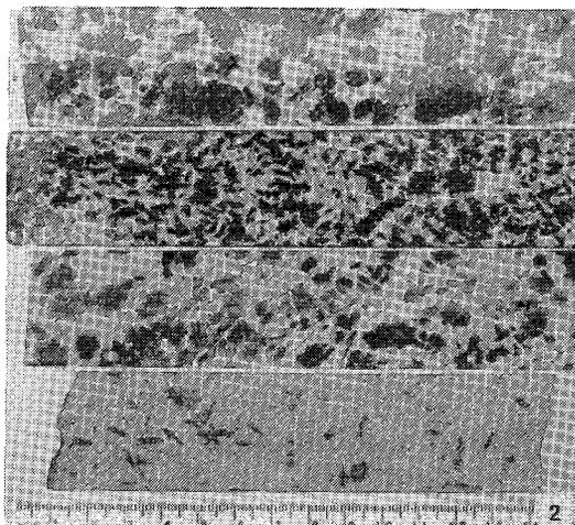
FIG. 2. Lizardite pseudomorphs after olivine (dark) in talc-carbonate (light). Diamond-drill-core samples. Scale in centimetres.
