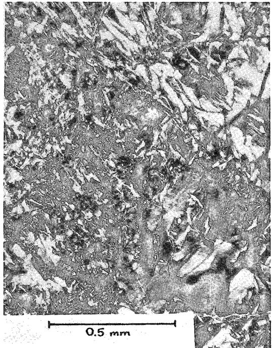
FIG. 6. Foliated texture of serpentinized dunite cumulate, showing replacement of lizardite of the early episode of serpentinization by antigorite of the late episode of serpentinization. Crossed nicols. Sample 1a–28578, Red Hills, Thetford Mines.
