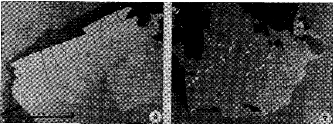
FIG. 6. Epoxy-mounted polished section of the crystal fragment ZH-5/10 of hafnian zircon showing prominent fracturing of the high-reflecting fresh subsurface zone (top), a slightly altered, darker, intermediate segment (centre) and dark metamict core (bottom). Note the veinlike spreading of the core-grade alteration into the intermediate segment, revealing fine growth-zoning by selective attack in initial stages. Also note the altered patches adjacent to, and in continuation of, the transversal cracks, restricted to the intermediate segment and not extending into the fresh subsurface zone.
