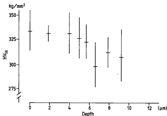
FIG. 1. The change in Vickers hardness,  $VH_{50}$  (in  $\text{kg}/\text{mm}^2$ ), with depth (in  $\mu\text{m}$ ) from the parting surface (0001) in pyrrhotite from Bodenmais. Sample S-1. Only undisturbed indentations were used for mean values.
