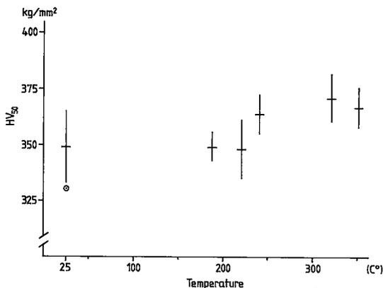
FIG. 3. The effect of annealing on the Vickers hardness in the parting surface (0001) in pyrrhotite. Circle: location of results from 100-gram-load tests. Only undisturbed indentations were used for mean values.
