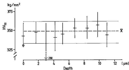
FIG. 2. The change in Vickers hardness with depth from the parting surface (0001) in pyrrhotite. Sample S-2. Dashed line: mean of all indentations made in this series. Upper and lower limit (limits of standard deviation) are indicated. Only undisturbed indentations were used for mean values. Circle indicates results of 100-gram tests.
