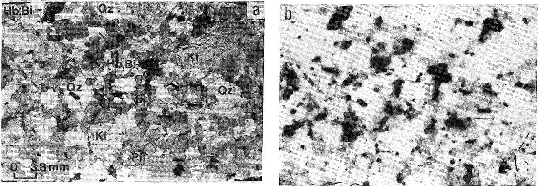
FIG. 3. Photomicrograph (a) and autoradiograph (b) of  $^{90}\text{Sr}$  sorbed on a sample of altered granite (Bi biotite, Hb hornblende, Kf microcline, Pl plagioclase, Qz quartz).
