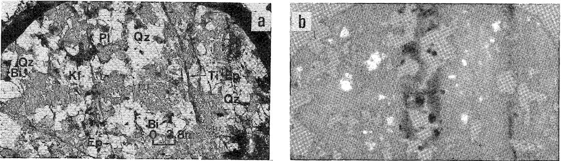
FIG. 7. Photomicrograph (a) and autoradiograph (b) of  $^{137}\text{Cs}$  sorbed on a sample of fractured granite. The matrix minerals adjacent to the microfractures are altered (Bi biotite, Ep epidote, Kf microcline, Pl plagioclase, Qz quartz, Ti titanite).
