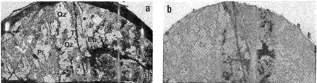
FIG. 8. Photomicrograph (a) and autoradiograph (b) of  $^{147}\text{Pm}$  sorbed from granite groundwater onto a sample of fractured granite (Ep epidote, Pl plagioclase, Qz quartz, Ti titanite). Note the preferential sorption of  $^{147}\text{Pm}$  on the fracture-filling materials.
