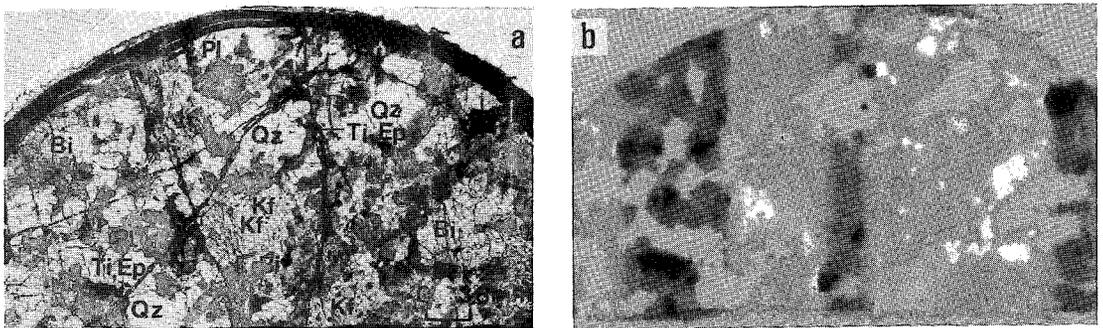
FIG. 6. Photomicrograph (a) and autoradiograph (b) of  $^{137}\text{Cs}$  sorbed on a sample of fractured granite. The matrix materials adjacent to the microfractures are altered (Bi biotite, Ep epidote, Kf microcline, Pl plagioclase, Qz quartz, Ti titanite).
