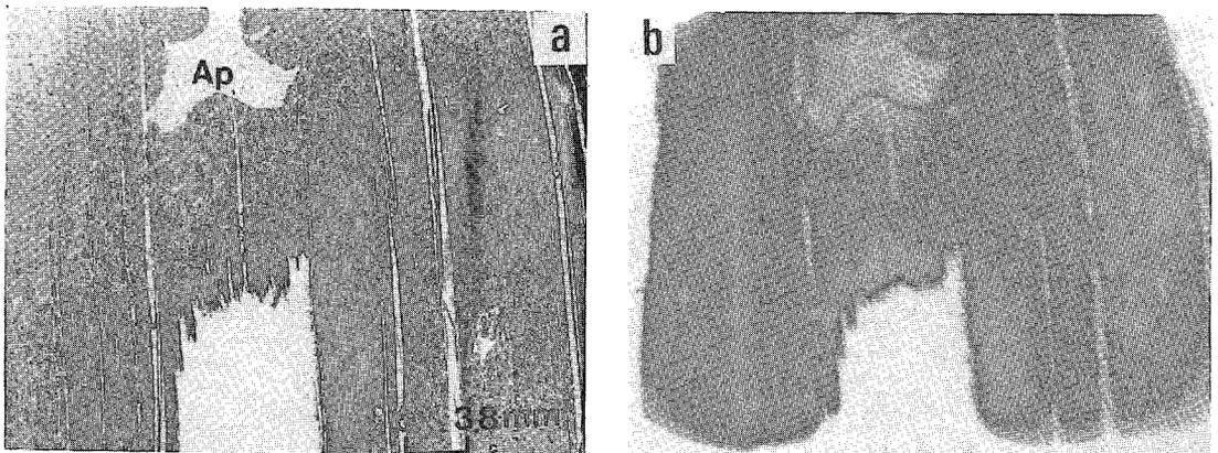
FIG. 10. Photomicrograph (a) and autoradiograph (b) of  $^{147}\text{Pm}$  sorbed on a thin section of biotite cut at  $45^\circ$  to the basal plane (Bi biotite, Ap apatite). Note strong sorption on the apatite inclusion.
