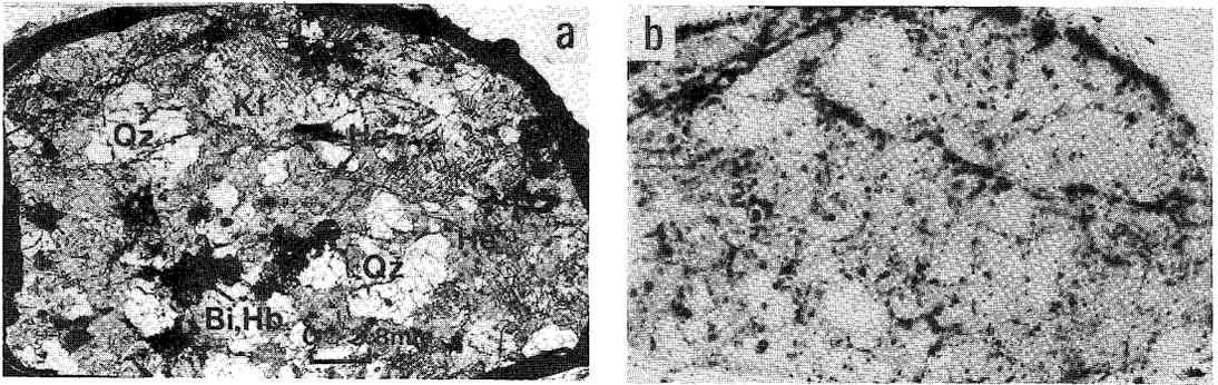
FIG. 13. Photomicrograph (a) and autoradiograph (b) of  $^{95m}\text{Tc}$  sorbed on a sample of fractured granite under anaerobic conditions (Bi biotite, Hb hornblende, He iron oxide, Qz quartz, Kf microcline). Note preferential sorption of  $^{95m}\text{Tc}$  on iron oxide fracture-filling material.
