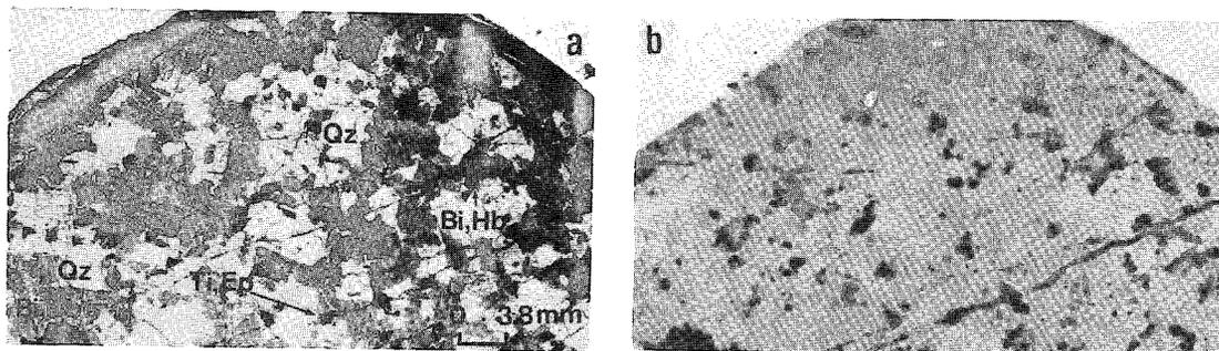
FIG. 12. Photomicrograph (a) and autoradiograph (b) of  $^{241}\text{Am}$  sorbed from a saline solution on a sample of fractured granite (Bi biotite, Ep epidote, Hb hornblende, Qz quartz, Ti titanite).
