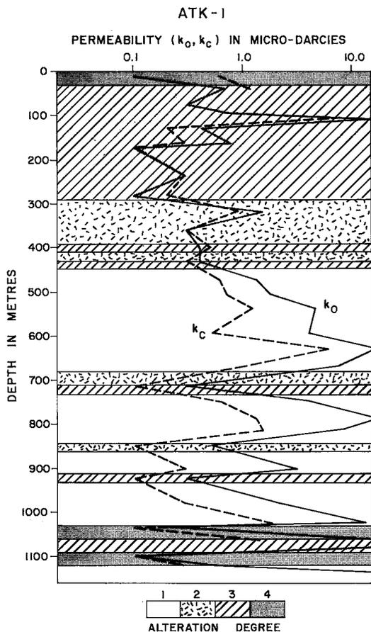
FIG. 5. Variation in hydraulic permeability  $k$  with depth and degree of alteration in the Atikokan research area;  $k_o$ ,  $k_c$  are hydraulic permeabilities measured under confining pressures of 1.4 MPa and equivalent overburden stress, respectively (after Katsube 1982).
