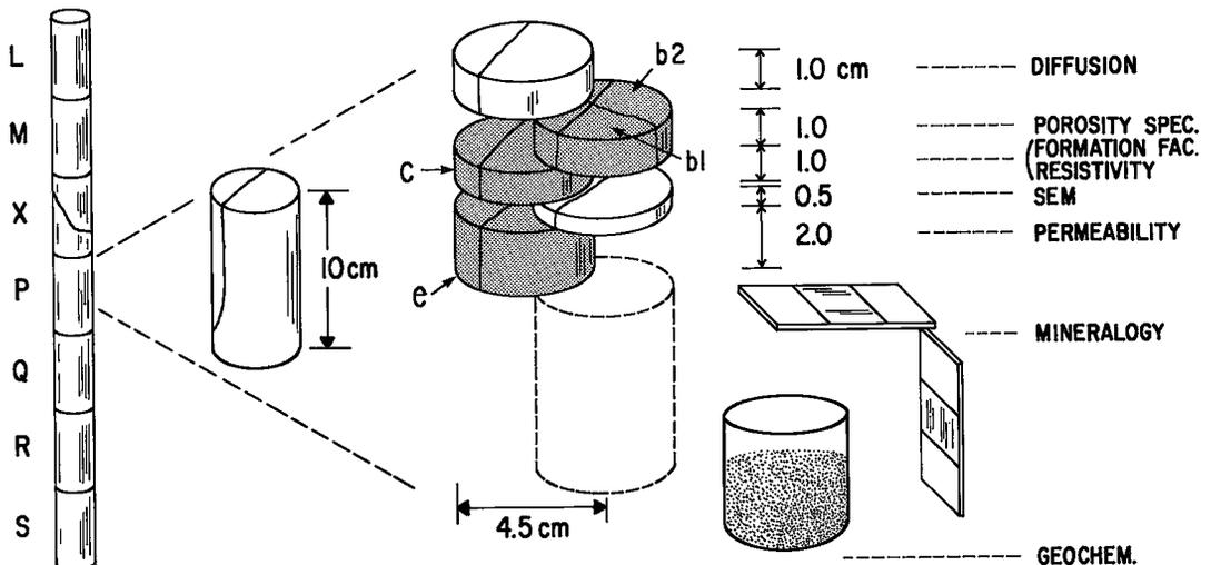
FIG. 3. Location of specimens within the sample and description of type of test performed on them.
