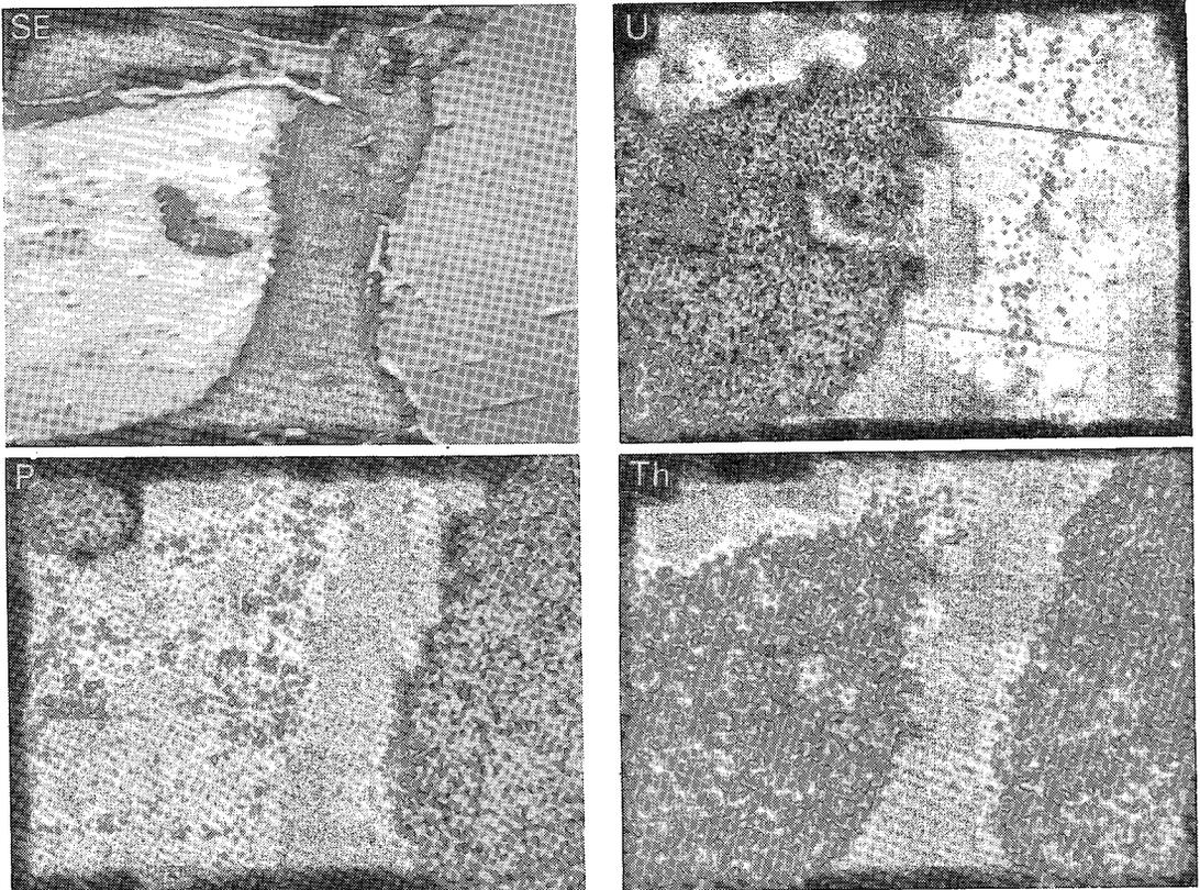
FIG. 2. Secondary-electron (SE), uranium (U), phosphorus (P) and thorium (Th) images of an unaltered "uraninite" (lower grain) and a monazite crystal (upper grain) in Karin Lake sample 72a. Width of field of view: 225  $\mu$ m.
