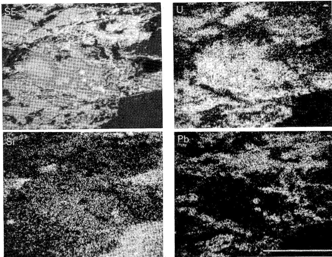
FIG. 4. Secondary-electron (SE), uranium (U), silicon (Si) and lead (Pb) images of extensively remobilized radioactive phases in a calc-silicate anatectite (sample 1010c) from the Spurjack Island area. Scale bar 100  $\mu\text{m}$ .
