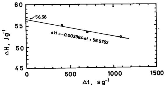
FIG. 3. Plot of  $\Delta t$  versus  $\Delta H$  for the cubanite transformation, intended to correct for the leakage of heat from the calorimeter. The formula of the regression line is shown. The corrected  $\Delta H$  is 56.58 J/g (sample).
