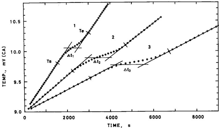
FIG. 2. Time-temperature plots to determine the transformation enthalpy of cubanite. On each plot, two regression lines, before and after the transformation, are drawn. The transformation period is shown between the two lines, in which  $T_s$  and  $T_e$  represent the starting and final temperatures, respectively. At the middle point between  $T_s$  and  $T_e$ , two regression lines determine the duration of the transformation  $\Delta t$ .
