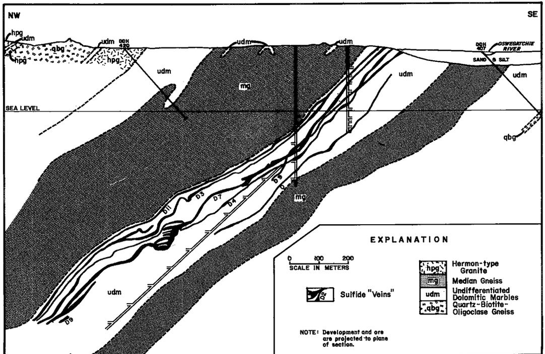
FIG. 2. Generalized geological section for the Edwards mine (modified from Lea & Dill 1968).
